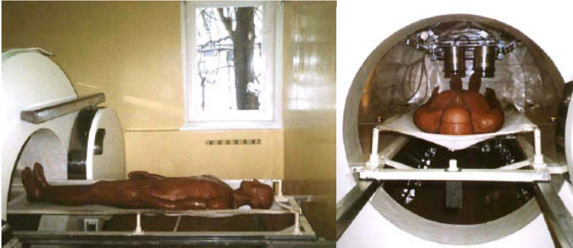
Fig. 3. Anthropomorphic phantom prepared to be measured.
