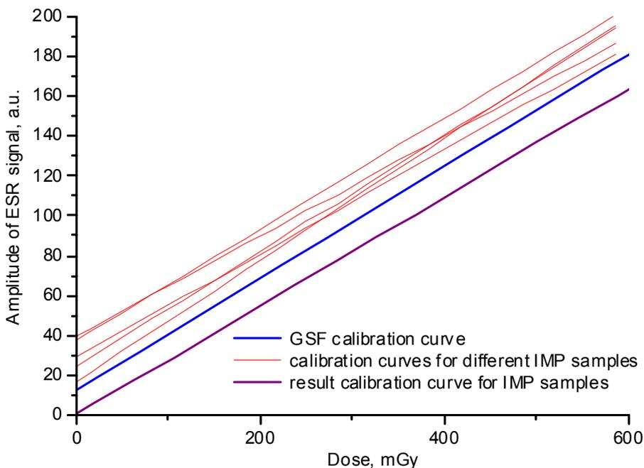
*Fig. A2. Comparison of the GSF- and the IMP-calibration curves.*
