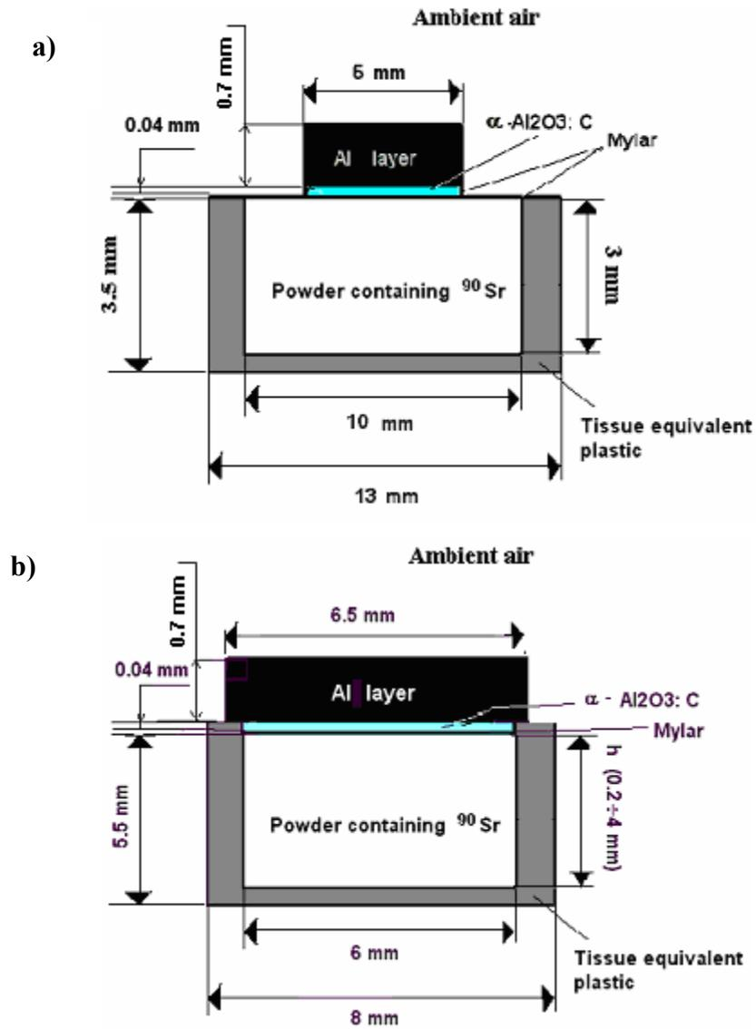
Fig. 24. Geometric description of simulation for detector calibration: a) initial geometry; b) new geometry.
