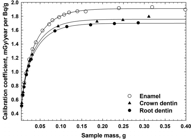
Fig. 26. The dependence of the calibration coefficient on sample mass in the new geometry. The symbols represent results of Monte Carlo simulations. The solid lines are fits to the data.
